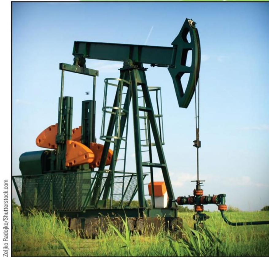
Figure 3.4: Small pump jack oil well.
