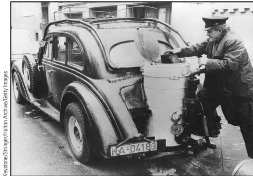
Figure 3.19: Automobile manufactured by Adler with wood gas generator attached to the back (Adler Diplomat equipped with Imbert Holzgas Generator, 1941).
